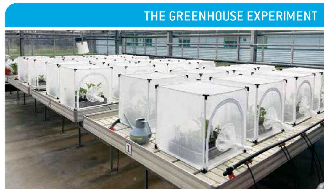
Set up of the greenhouse experiment where plants were inoculated with different combinations of BMV, BChV, BYV and BtMV. The plants were kept in the tents during the whole experiment to avoid contamination.
